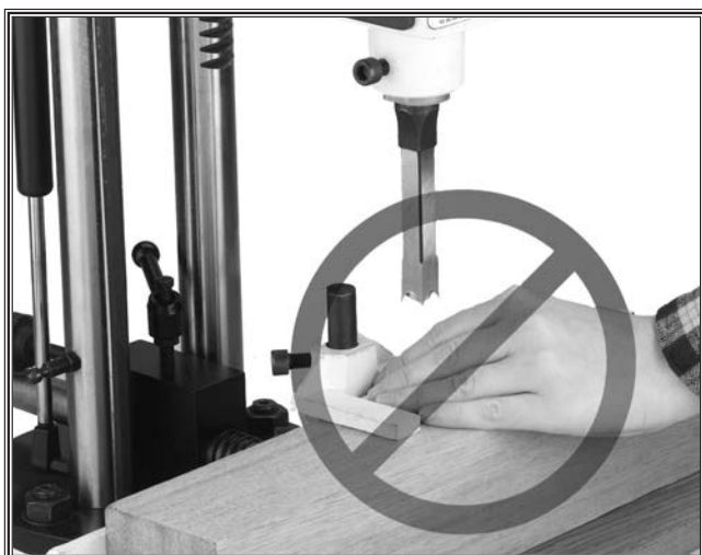
Figure 5. Never place hands under chisel.
