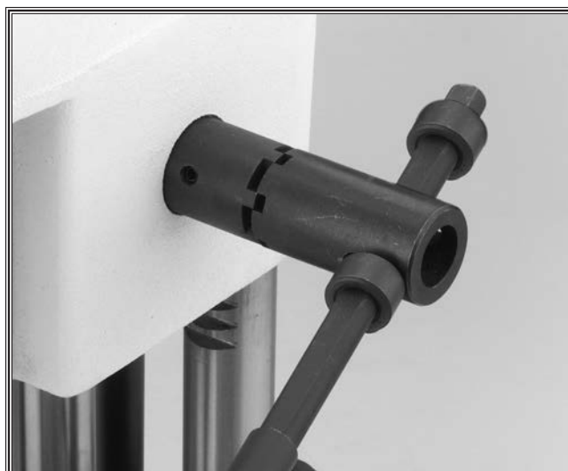
Figure 16. Indexing handle by swinging out.
