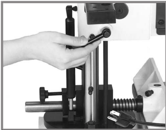
Fig. 4. Secure depth stop before removing gas spring.
