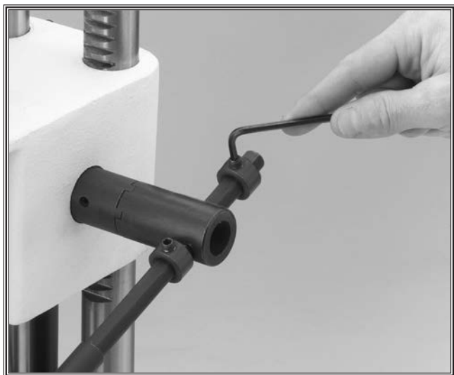
Figure 15. Secure collar onto hand lever.
