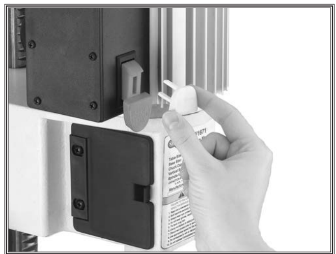
Figure 7. Remove safety key when not in use.
