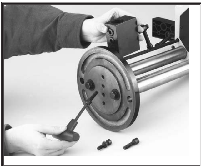
Figure 32. Repositioning the support block.
