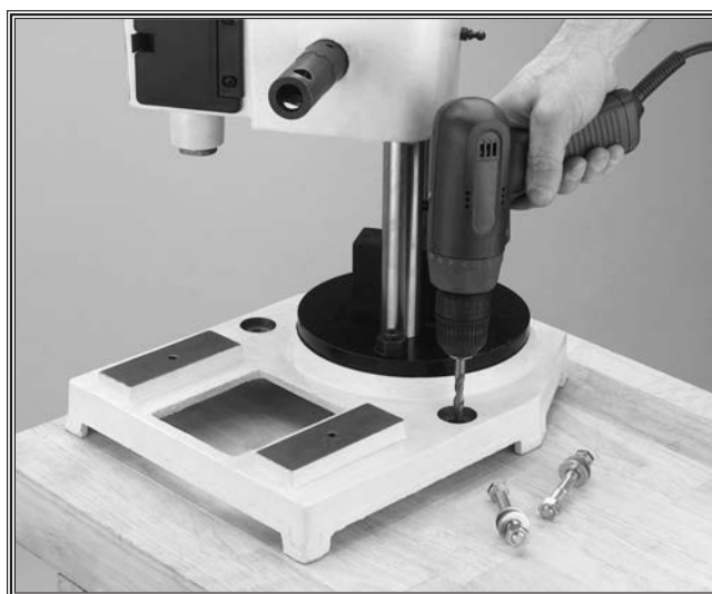
Figure 13. Using mounting holes as drill guides.
