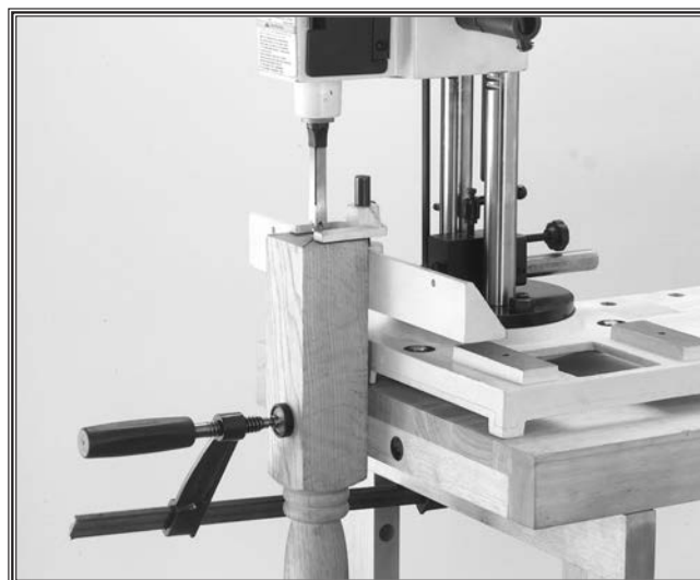
Figure 28. Workpiece clamped to edge of table.
