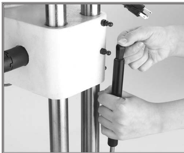
Figure 17. Compressing gas spring to assemble.
