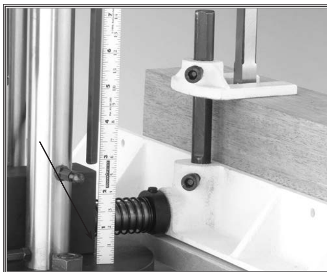
Figure 35. Setting the depth stop to 2\frac{7}{8} ".
