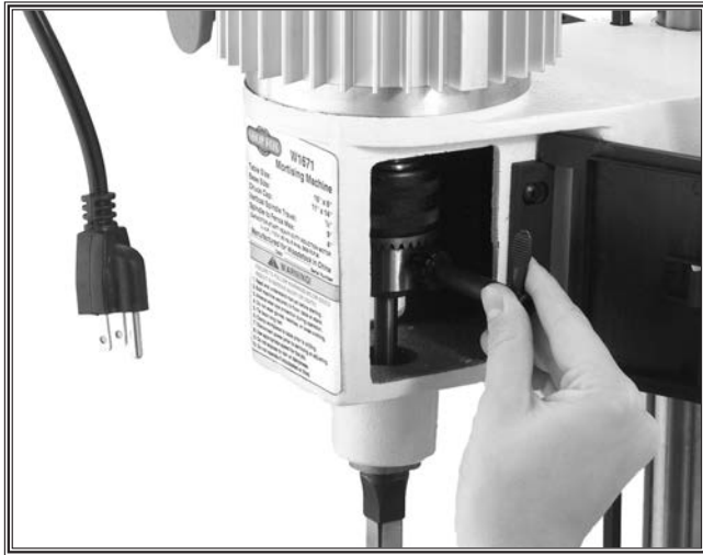
Figure 3. Unplug before changing chisels.
