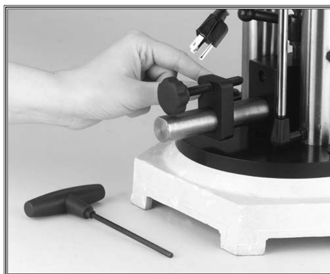
Figure 30. Setting micro-adjusting block.
