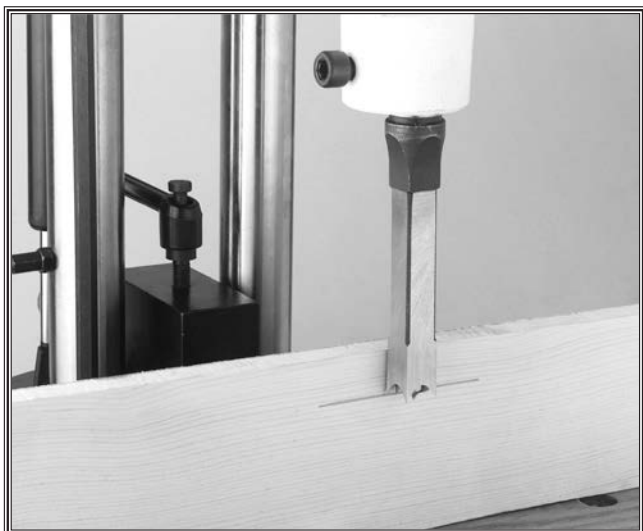
Figure 36. Use penciled line to gauge depth.
