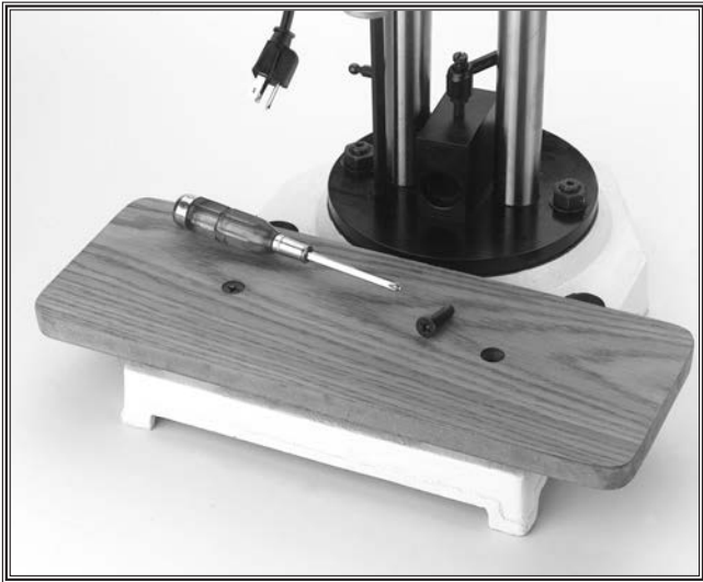
Figure 18. Work table secured with screws.
